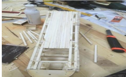
Fig. 14. Reinforcements of the Lower Bridge Structure
