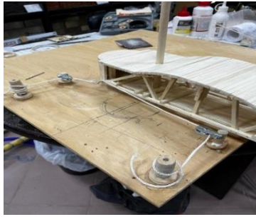
Fig. 16. Complete Rotational System with Axis
